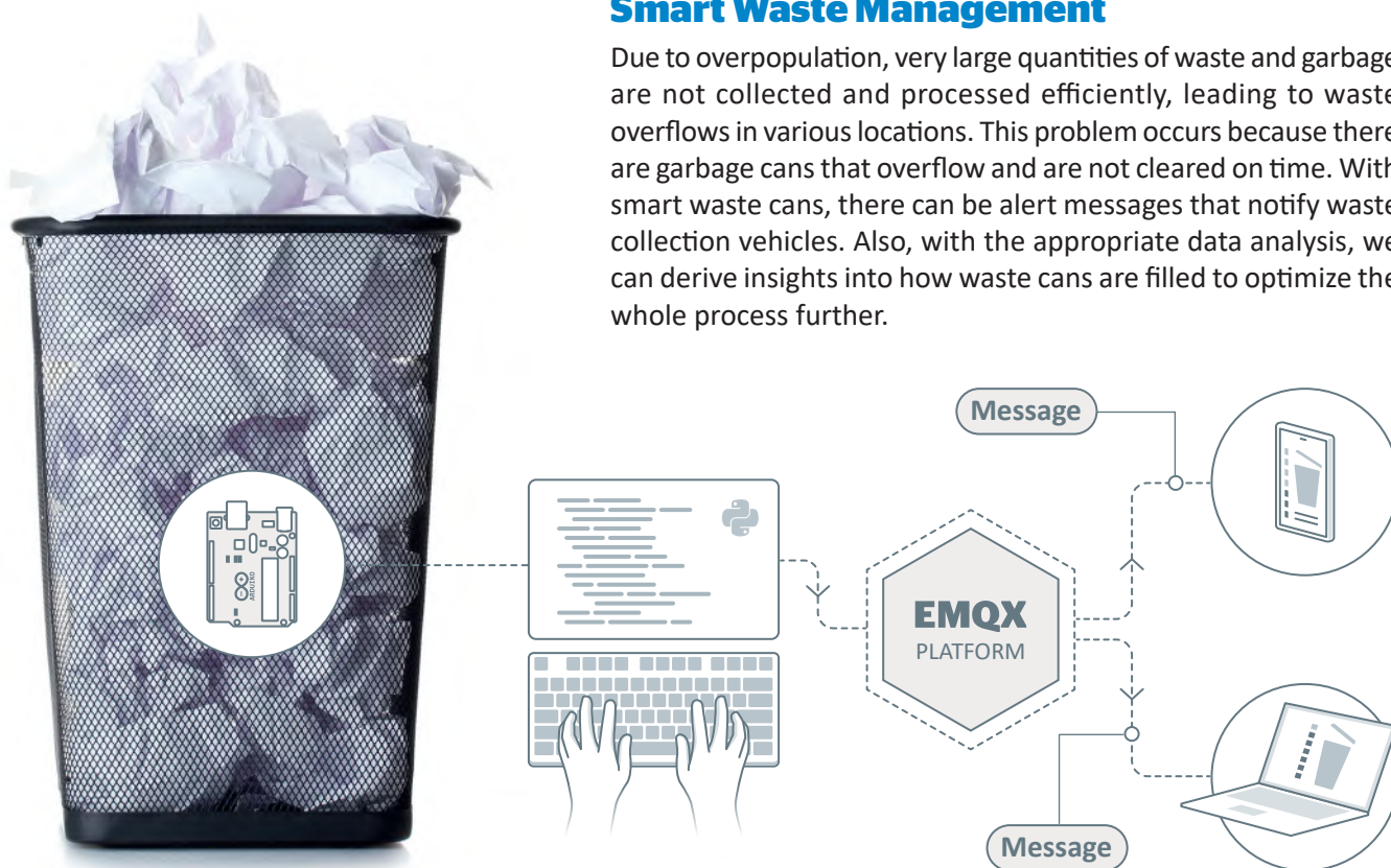
Figure 3.8: Smart Waste Management Arduino & MQTT project
